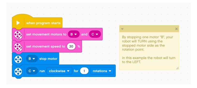
TEST IT: Experiment with the other motor
