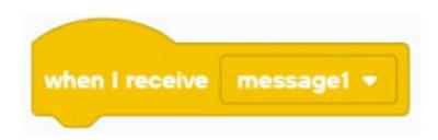
When I Receive Message BLOCK Runs the blocks attached to it when a specific message is broadcasted by either the Broadcast Messsage or the Broadcast Message and Wait Block.
