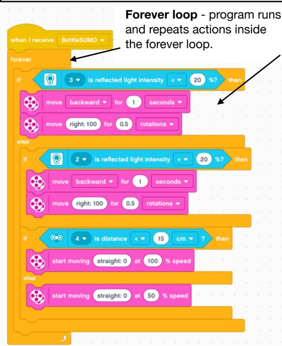
The robot looks for the bottle with the Ultrasonic sensor WHILE checking to see if it's on or off the table using the colour sensors.
