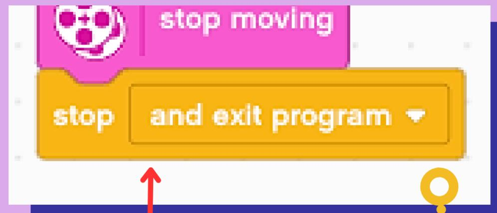
Add this stop block and select 'and exit program' to tell the robot to stop running the program after all the previous actions have occurred.
